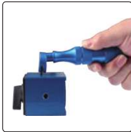
step 1: make grid cutting on surface
